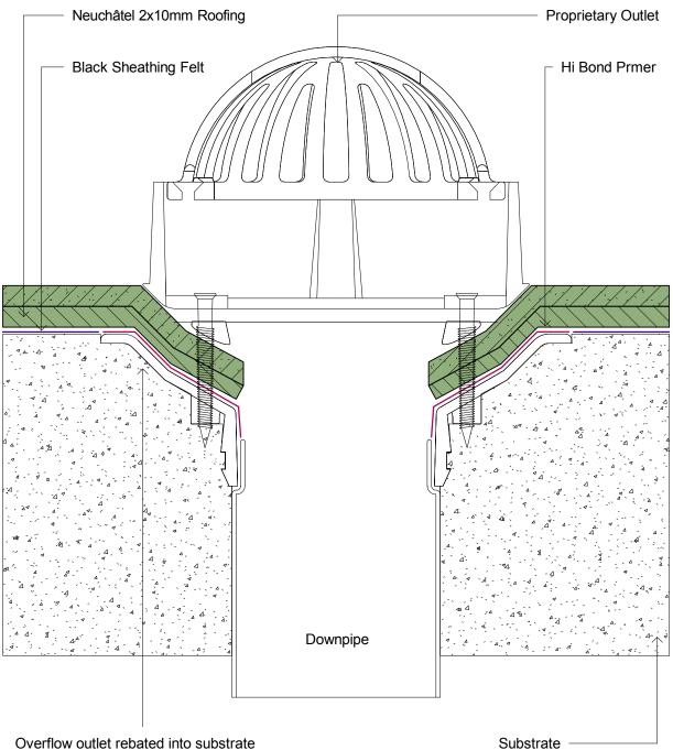
Overflow outlet rebated into substrate and screwed into place with S/S screws
