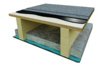
Timber joists supporting plywood panels. In the past tongued and grooved timber boarding or chipboard were used. Neuchâtel waterproofing systems (built-up bitumen felt, Neuchâtel Asphalte, single ply membranes) are installed (using various means of attachment) to the top of the timber deck. Foil backed plasterboard to the soffit, with fibreglass insulation above and an air space above the insulation.
