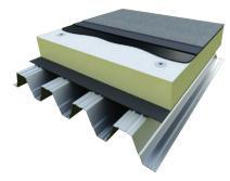
There are three preferred structural decks, concrete, timber (plywood) and the most popular being profiled galvanised metal deck on steel purlins. These deck systems are usually installed flat. Metal decking and plywood could be installed to falls at extra cost.
