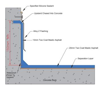
Cast concrete up stand detail
