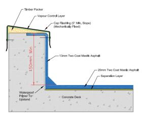
CAST CONCRETE PARAPET WITH CAP FLASHING
