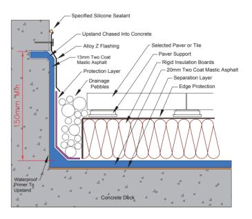
Neuchâtel Mastic Asphalt inverted insulated roof X-sectional
