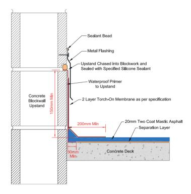
Neuchâtel green roof/concrete up stand/edge trim X-sectional detail
