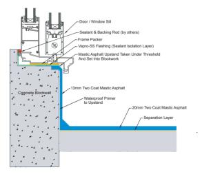
**BLOCKWALL THRESHOLD UPSTAND DETAIL**
