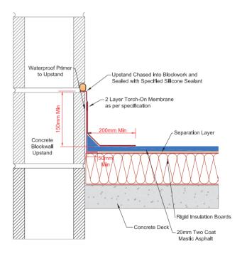
Neuchâtel Mastic Asphalt insulated car park - roof X-sectional detail
