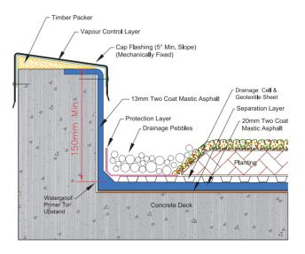
Neuchâtel Mastic Asphalt green roof/concrete up stand/cap flash-
