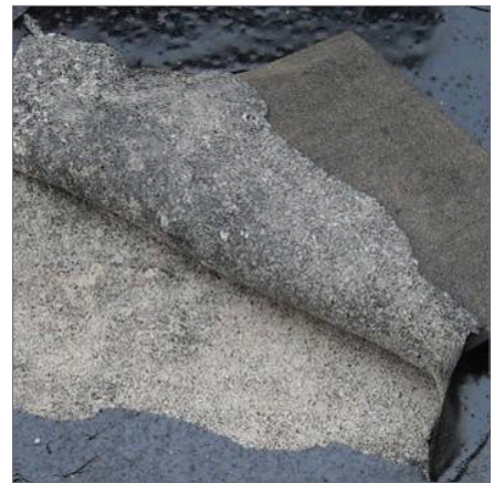
Failed peel - easily pulled from the substrate
