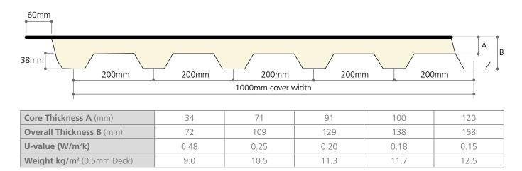
**Note:** IKO Spectradek insulated roof panels have a thermal transmittance (U-value) as detailed in the table above, calculated using the method required by the building regulations Part L2 (England & Wales) and Building Standards Section 6 (Scotland).
