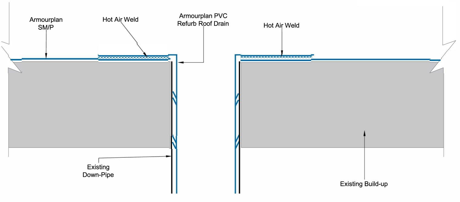
Fixing to existing roof substrate will require core sample to be taken and pull out test will be required to establish suitability of the roof deck
