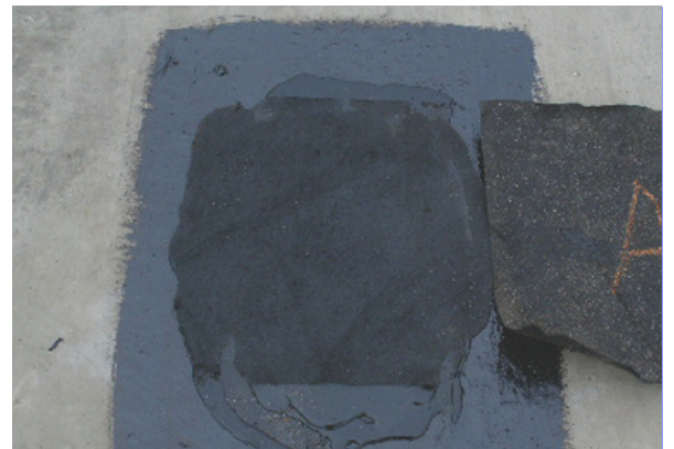
Successful peel test example
